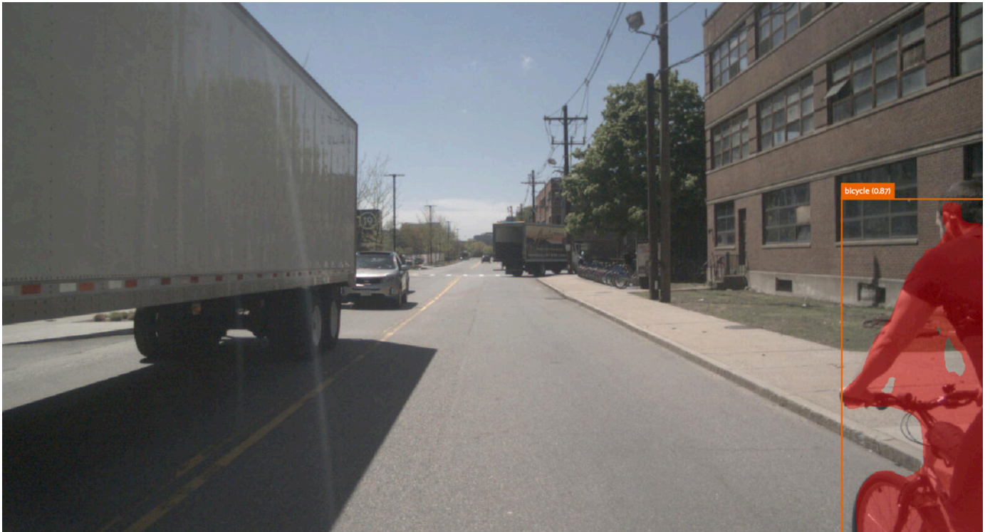
Figure 10 d): The model pre-trained on synthetic data detects a partially occluded cyclist at a close distance from the ego.
