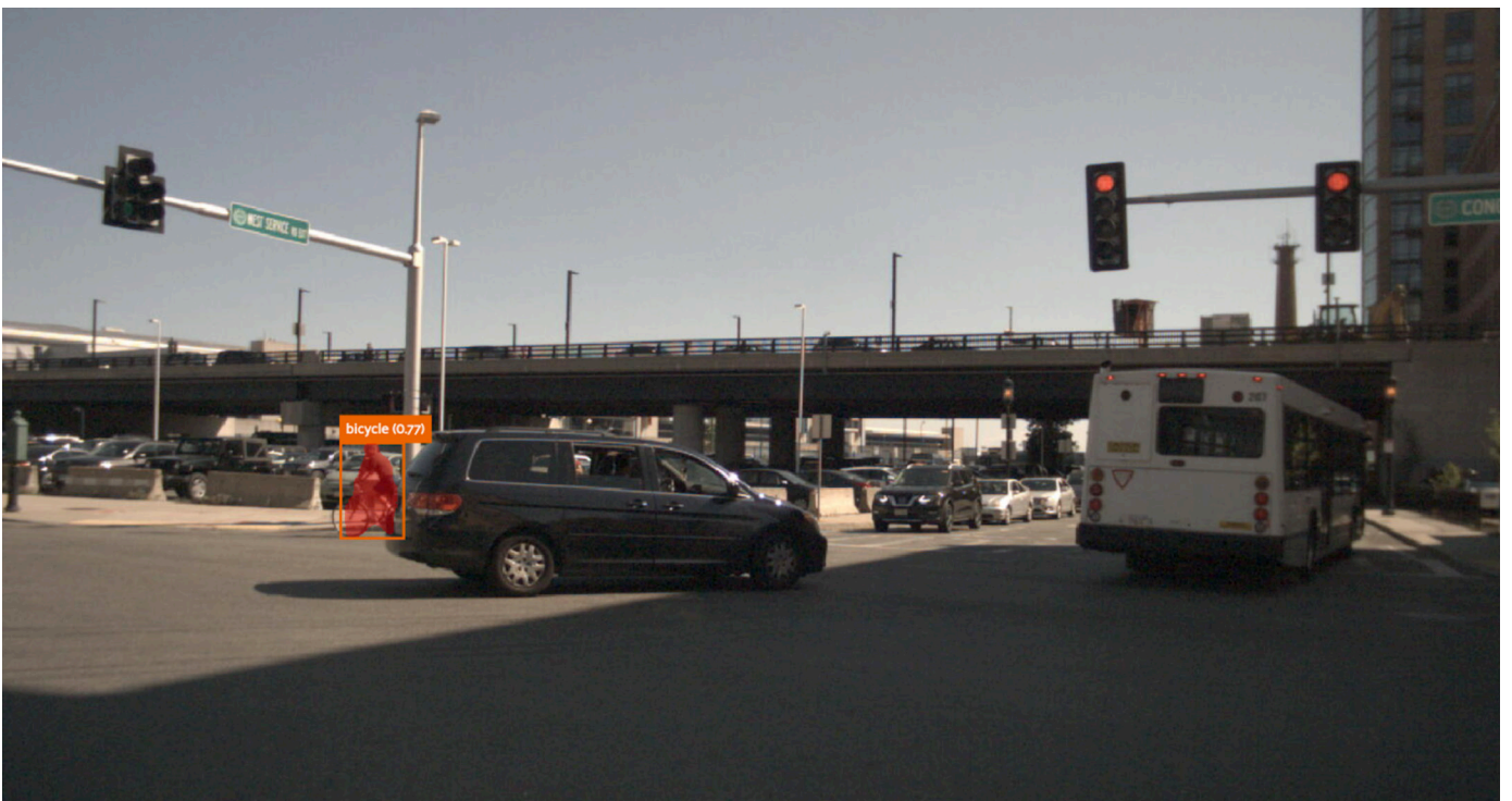
Figure 10 e): The model pre-trained on synthetic data detects a partially occluded cyclist at a distance.
